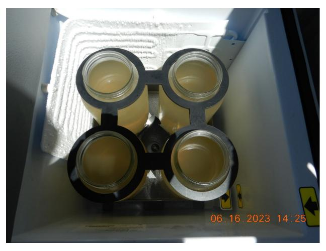
Photo A-2. Sample jars in refrigerated autosampler at Building 132
